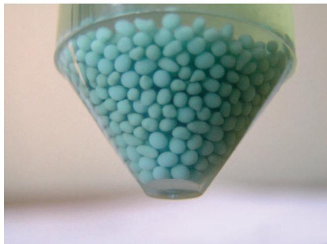
Figure 2. Mixed copper-loaded alginate/chitosan capsules
