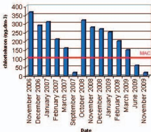
Figure 7. Fluctuation of chlortoluron concentration in drainage water for drainpipe spacing of 15 m
