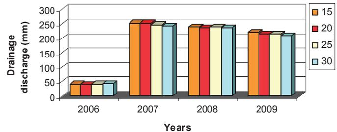
**Figure 3.** Quantities of drainage discharge (mm) for different drainpipe spacing
