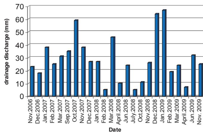
Figure 5. Fluctuation of drainage discharge (mm) for drainpipe spacing of 15 m
