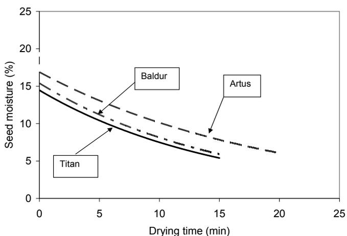
Figure 3. Drying curves for investigated hybrids at air temperature of 80 °C
