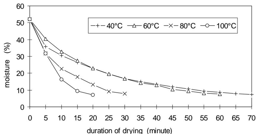
Graph 2. Drying of pumpkin seeds at the airflow speed of 1.2 m/s
