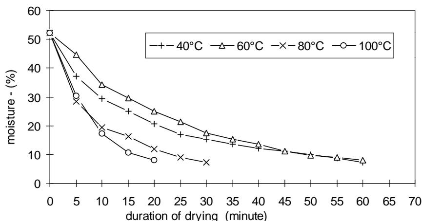
Graph 3. Drying of pumpkin seeds at the airflow speed of 1.6 m/s
