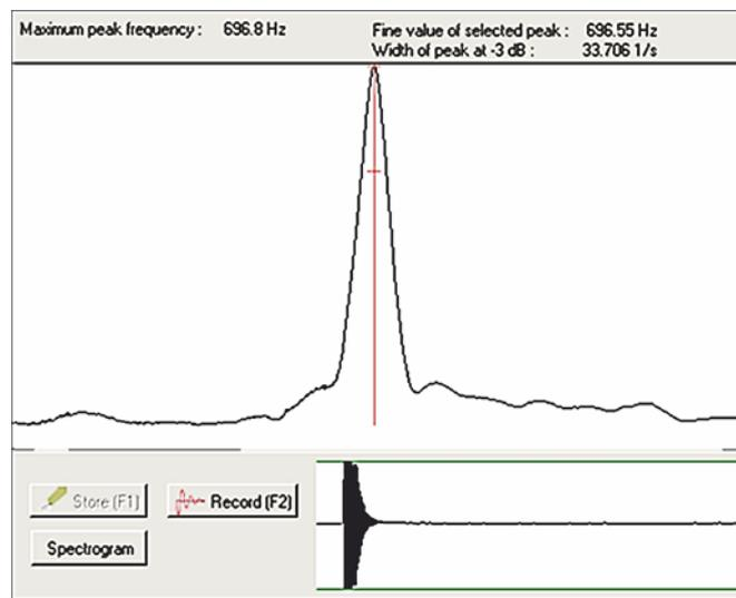
**Figure 1.** Typical Appearance of the processed acoustic signal of 'Gloster' apple obtained by "Stiffness" software. (Lower curve shows the apple fruit's recorded acoustic response. Upper curve shows appearance of the apple fruit's acoustic frequency spectrum. The resonant frequency of the highest peak (with the largest wave amplitude) and its width at the upper third of its height are shown numerically at the top of the picture)
