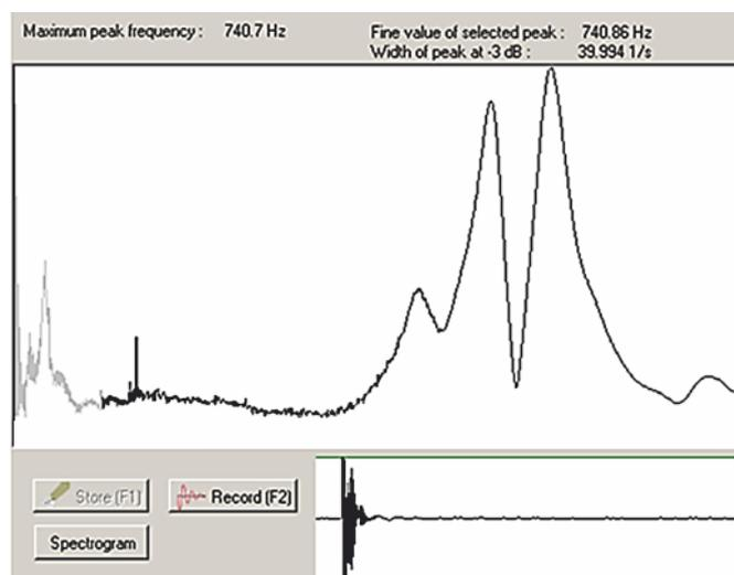
Figure 2. A typical acoustic signal with two peaks of similar height of 'Gloster' apple obtained by "Stiffness" software
