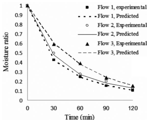
Figure 3. Variation of experimental and predicted moisture ratio versus drying period at three levels of flow rate for 30° of the collector inclination angle
