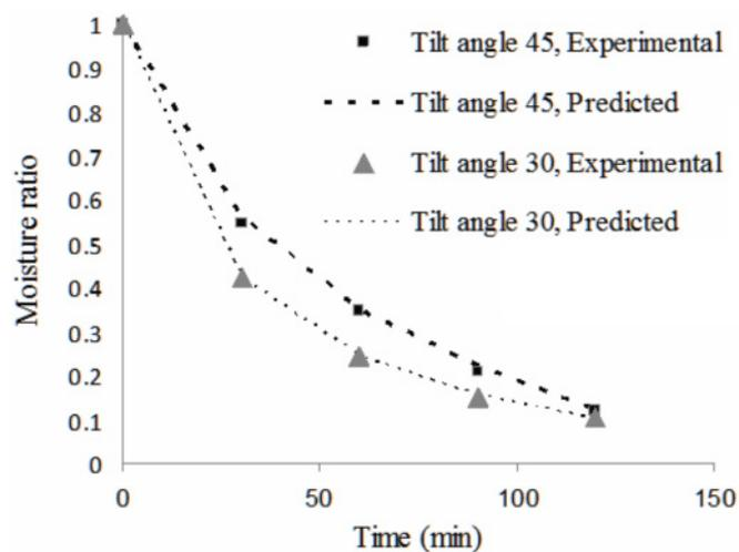
Figure 5. Comparison between moisture ratio variations in different inclination of the collector
