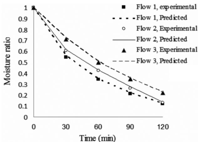
Figure 4. Variation of experimental and predicted moisture ratio versus drying period at three levels of flow rate for 45° of the collector inclination angle
