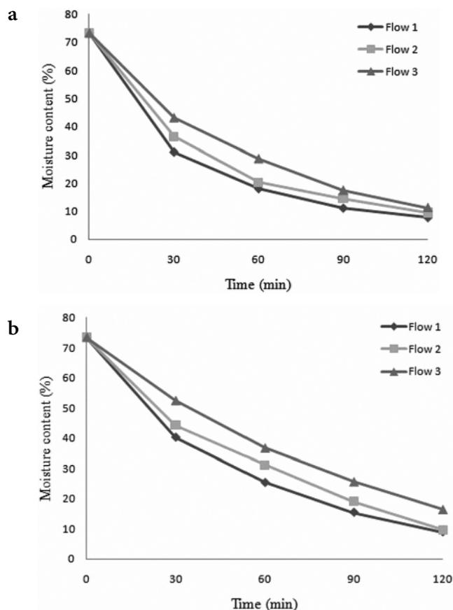
Figure 2. Variations of experimental moisture content versus drying time for apple at three airflow rate and collector tilted angle (a: 30° and b: 45°)
