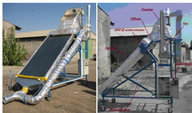
Figure 1. Solar dryer components
