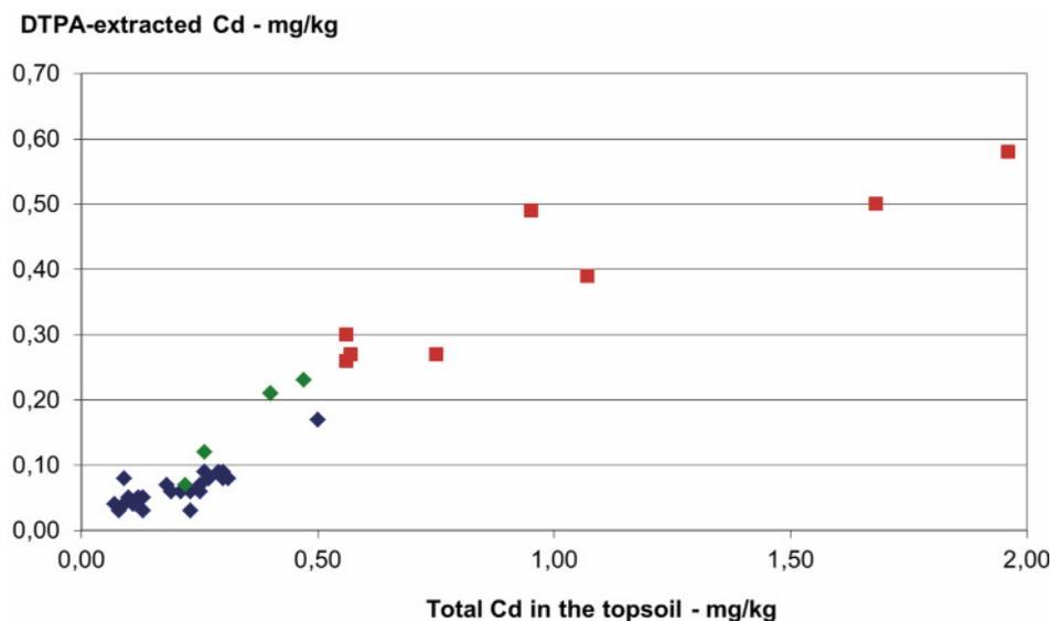
Figure 4. Soils of the Limoges area (36 ploughed horizons). Relationship between cadmium extracted with DTPA and total Cd in topsoil samples. “Large quantities” sites are shown by red squares, “moderate quantities” by green diamonds and “small quantities” and control sites by blue diamonds (Courbe et al., 2002)
