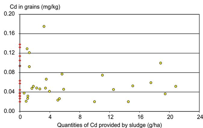
**Figure 6.** Trials in Burgundy and Franche-Comté (Deléan and Kockmann, 2003). Relationship between cadmium content in wheat grains and Cd quantities provided by sewage sludge application ( $R^2 = -0.016$ ). Cadmium-input in 15 control plots are nil.
