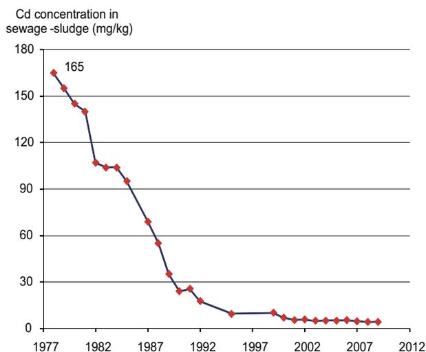
**Figure 1.** Mean annual cadmium concentrations from 1978 to 2009 in sludge from the treatment plant of waste-waters of Greater Paris (at Achères). This concentration has decreased strongly over time from 160 to 4.3 mg kg<sup>-1</sup> DM
