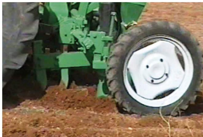
Figure 2. Mulch injection into soil by the machine
