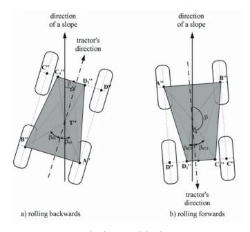
Figure 2. Longitudinal static stability limit
