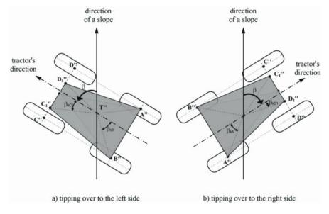
Figure 3. Lateral static stability limit
