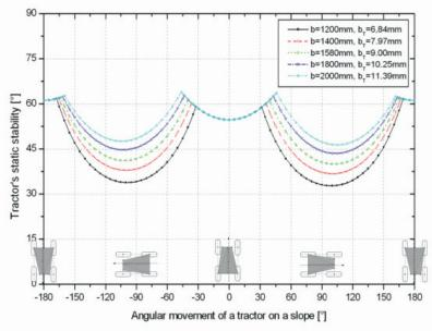
Figure 7. Simulating tractor's static stability in relation to the changes of the track width
