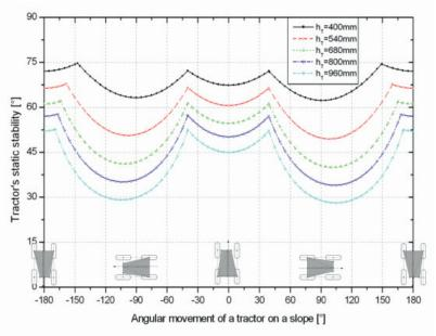
Figure 11. Simulating tractor's static stability in relation to the changes of the distance between the centre of gravity and the ground
