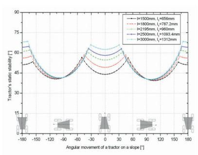
Figure 6. Simulating tractor's static stability in relation to the changes of the wheelbase
