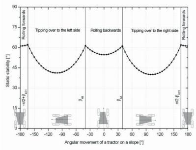
Figure 5. Simulating static stability of the Reform MOUNTY 65 mountain tractor
