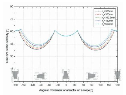
**Figure 8.** Simulating tractor's static stability in relation to the changes of the height of the front axle mounting point
