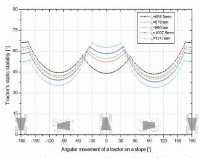
**Figure 9.** Simulating tractor's static stability in relation to the changes of the distance between the centre of gravity and the rear axle
