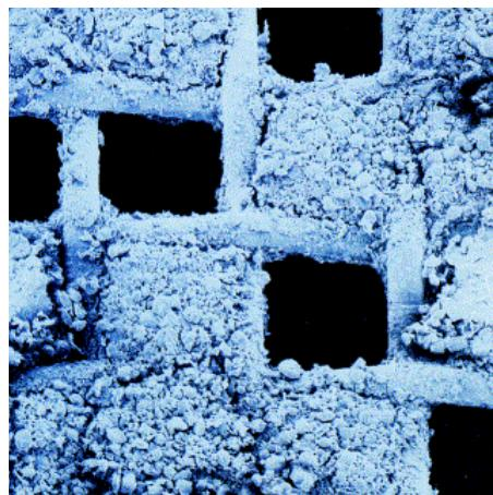
Figure 1. Sieve blocked with agglomerates (O'Connell, 2003)
