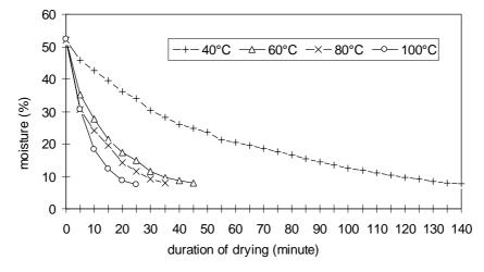
Graph 1. Drying of pumpkin seeds at the airflow speed of 0.8 m/s
