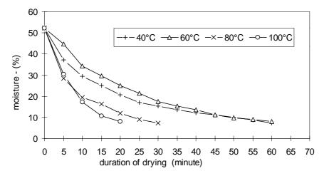
Graph 3. Drying of pumpkin seeds at the airflow speed of 1.6 m/s
