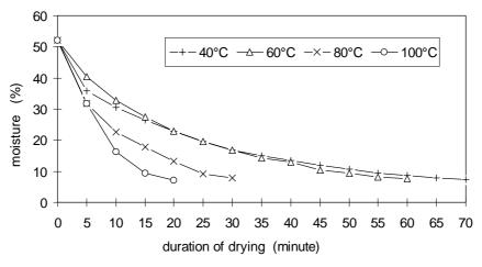
Graph 2. Drying of pumpkin seeds at the airflow speed of 1.2 m/s
