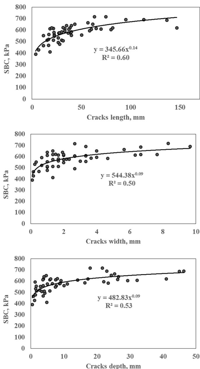
**Figure 7.** The relationship between length, width and maximum depth of soil cracks with soil bearing capacity (SBC) at harvesting time
