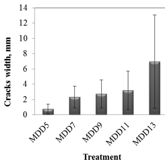
**Figure 5.** Width of cracks created on soil surface in different mid-season drainage duration (MDD) treatments
