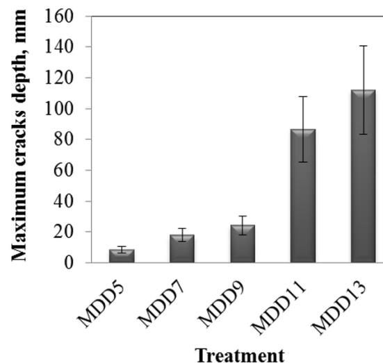
**Figure 6.** Maximum depth of cracks created on soil surface in different mid-season drainage duration (MDD) treatments
