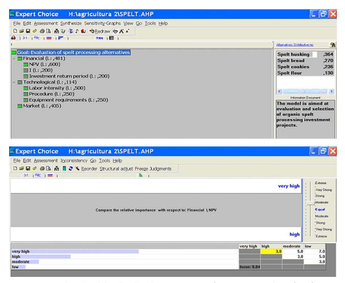
Figure 3. AHP hierarchy with derived weights and pair-wise comparison of intensities in Expert Choice software for financial attribute 'Net present value'
