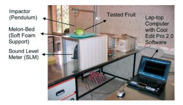
Figure 2. Setup of experiment for acoustic impact test
