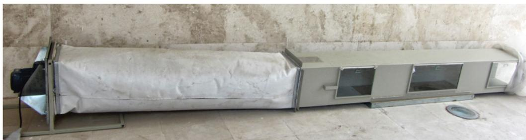
Figure 2. Wind erosion meter
